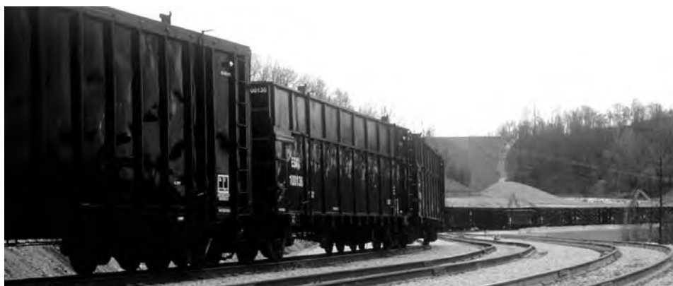
ESIX covered gons spotted for unloading on new spur to landfill.
